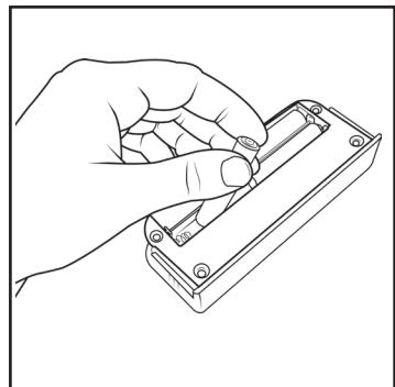
2. Insert 4 AAA batteries into the light. Ensure the batteries are inserted so that the flat ends are making contact with the springs.
