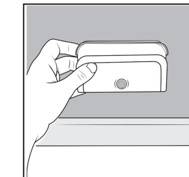
3. Slide the light onto the mounting plate. When changing batteries, slide the light off the mounting plate to access the battery compartment.
