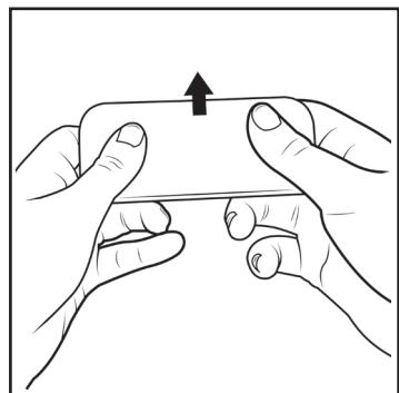
1. Remove the mounting plate from the back of the light by sliding the mounting plate up.
