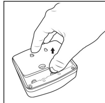
2. Use the tab on the battery door to lift up. If the door is too tight to lift with your fingers, use a flat head screwdriver.
