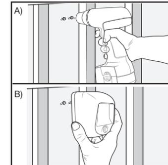
2. A) Use a 1/16" drill bit to create the pilot holes. Drill the screws into the pilot holes, leaving 1/4 inch of space between the screw and the surface. B) Slide the light onto the screws by lining up the screws with the keyholes on the battery cover.
