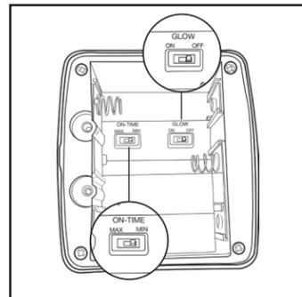
3. Before inserting the batteries, choose your On-Time and GlowMode™ settings. The maximum On-Time is 60 seconds after motion stops and the minimum is 20 seconds. If you set GlowMode™ to ON, a low light will stay on continuously at night.
