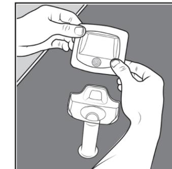
4. Slide the bracket and the light into the stake.
