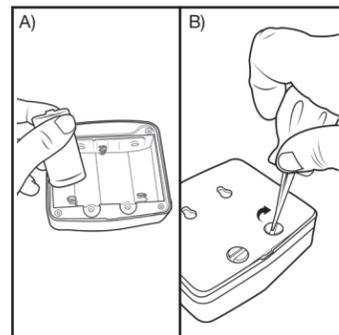
4. A) Insert 3 C-cell batteries into the light. Before replacing the battery cover, follow step 1 in the light installation instructions. B) Replace the battery cover by turning the screws clockwise until the lid is completely shut.
