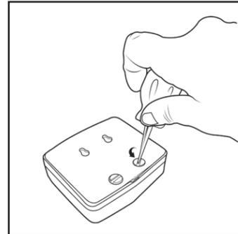
1. Remove the battery cover from the light by taking out the screws. Twist the screws counterclockwise until they are completely removed. Set aside.
