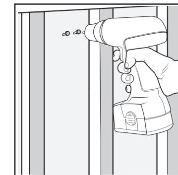
2. Use a 1/16" drill bit to create the pilot holes. Drill the screws into the pilot holes, leaving 1/4 inch of space between the screw and the surface.
