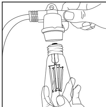
1. Ensure the bulb is compatible with the cord based on the wattage and socket type. See chart above for specs.
