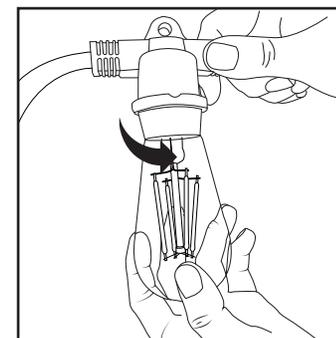
2. Unplug the string light cord, then screw the bulb into the socket.\*
