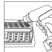
3. Place the light in the desired mounting location and drill the screws through the holes at the top of the light to secure the light into place.
