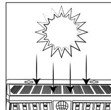
2. Determine the mounting location. We recommend a mounting height of 6.5-8 feet in an area that receives direct sunlight.
