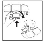
3. If mounting to an eave, the motion sensor must be positioned in front of the light heads (as shown above) for optimum motion detection. Before mounting, with the light facing you and the sensor centered and at the bottom, push the sensor up and rotate it 180 degrees so the dials are facing up.
