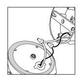
**4.** Pair the white (neutral) wire from the junction box with the white (neutral) wire from the light fixture and connect the ends with a wire nut (D). Pair the black (live) wire from the junction box with the black (live) wire from the light fixture and connect the ends. with a wire nut.
