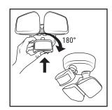
3. If mounting to an eave, the motion sensor must be positioned in front of the light heads (as shown above) for optimum motion detection. Before mounting, with the light facing you and the sensor centered and at the bottom, push the sensor up and rotate it 180 degrees so the dials are facing up.
