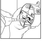
2. Insert one mounting bracket screw (B) on each end of the bracket with a Philips screwdriver.
