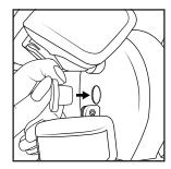
**6.** Insert the silicone cap (E) into the screw hole. Use appropriate exterior silicone sealant to seal around the outside of the fixture between the canopy and the house.
