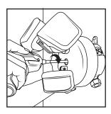
5. Align the light fixture's base to the junction box. Put the mounting screw (C) through the hole in the center of the fixture, and drive the screw through the center hole of the mounting bracket. Be sure that the wires are not pinched during this step.
