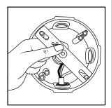
1. Cut power to the junction box by turning off the power breaker. Confirm there is no power by using a voltage tester. Align the mounting bracket (A) to the screw holes in the junction box.
